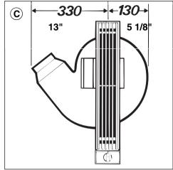
■ An opening of at least 135 mm (5-5/16") diameter must be cut in the kitchen cabinet in order to allow the exhaust ducting to pass through.
